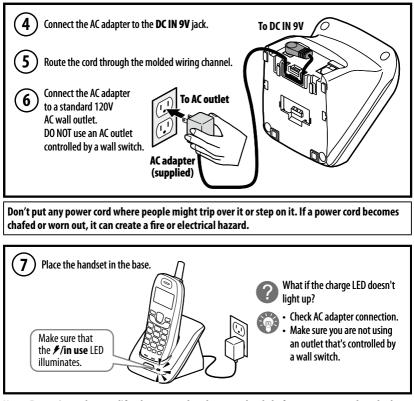
Note: For optimum battery life, charge your handset completely before you connect the telephone cord. The first time you charge a new battery, allow 15 to 20 hours.
